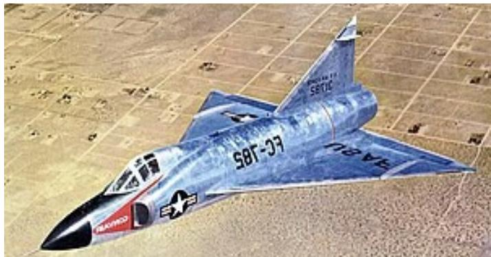
The **Convair F-102 Delta Dagger** is an interceptor aircraft designed and produced by the American aircraft manufacturer Convair. A member of the Century Series, the F-102 was the first operational supersonic interceptor and delta-wing fighter operated by the USAF.
